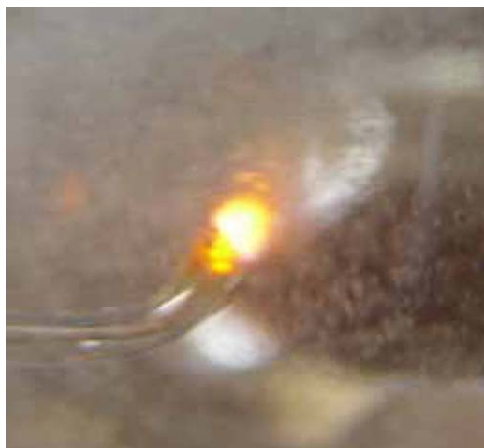
Fig. 3. Photograph of glow discharges at 600 V in aqueous solution.
